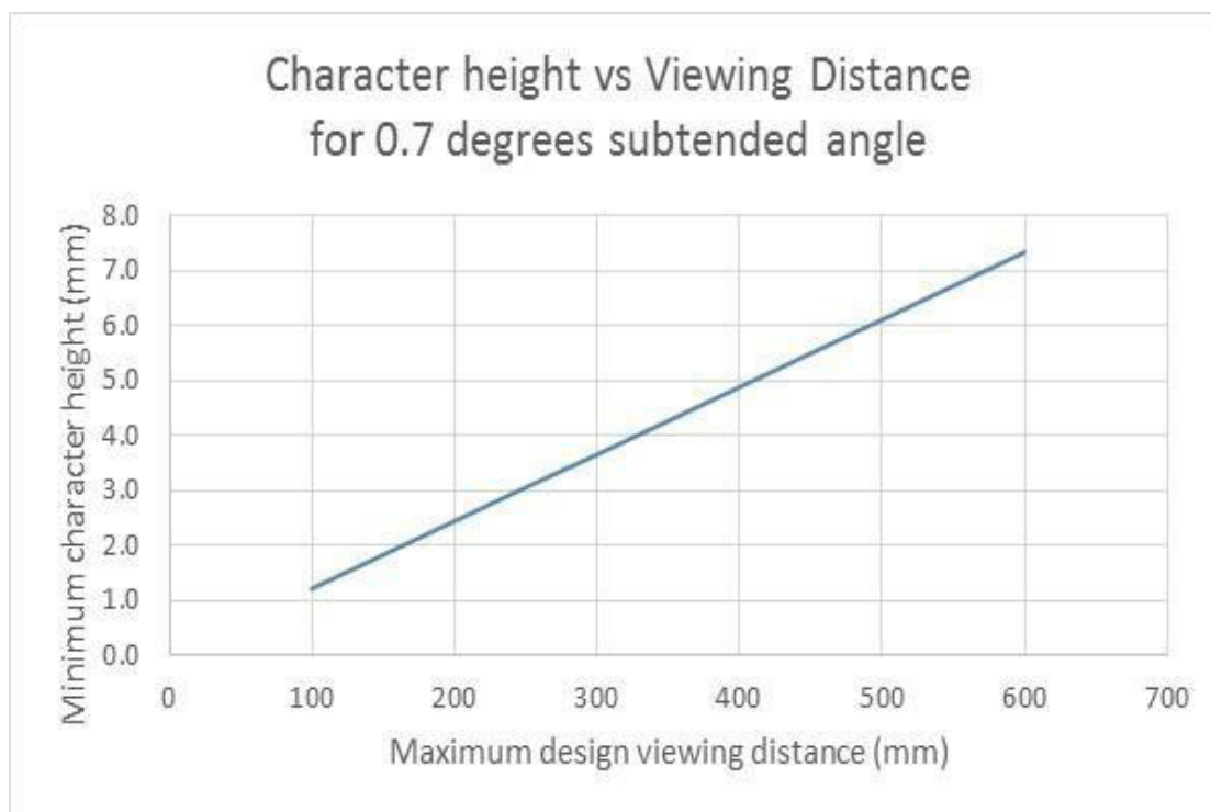
FIG. 1 RELATIONSHIP BETWEEN MINIMUM CHARACTER HEIGHT AND MAXIMUM DESIGN VIEWING DISTANCE
